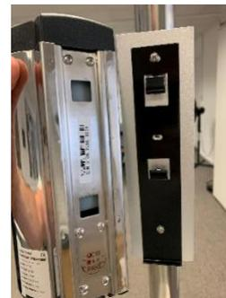
6. Take Sanillo dispenser from box and remove Black rectangular fixing panel and attach to mounting plate on the pole, ensuring it is attached the correct way up. Insert and tighten top screw with locking washer first, and then the bottom hole will then line up for securing to the corresponding hole in the back plate
